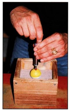
Soil testing laboratories perform a penetrometer test to measure a sand's resistance to compression. The value from this test is used to predict the sand's potential for fried-egg lies.
