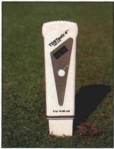
New, low-cost meters are available to help superintendents better manage their courses. The TDSTestr 4™ meter measures salt accumulation in the root zone from saline irrigation supplies and lets superintendents know when overirrigation is required to prevent turf damage.
