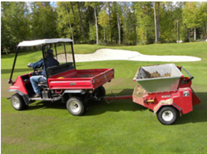
In the world of golf course maintenance, utility vehicles are the “jacks of all trades” as they can be used throughout the day transporting crew members, hauling tools or materials, or even operating other equipment like this small topdresser.
