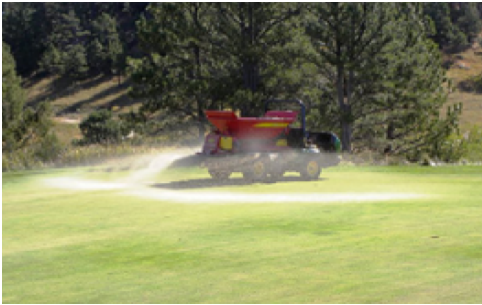
A large capacity, twin spinner-type topdresser applies sand at a light rate over a putting green.
