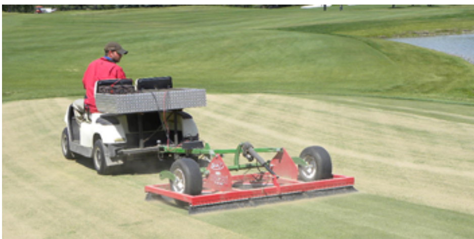
When it comes to topdressing equipment, many golfers don't think about other equipment needed such as this drag broom to sweep sand into the turf canopy of a putting green.
