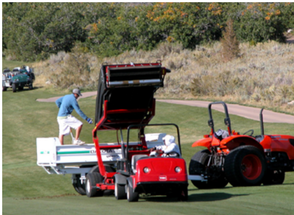
Major cultivation practices require multiple pieces of equipment. Here, for the cleanup of aeration cores from fairways, a heavy-duty utility vehicle operates a sweeper that empties the collected soil cores into a large material hauler trailer pulled by a tractor.
