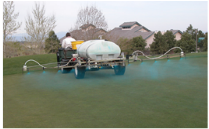
Modern sprayers have numerous features and options to maximize the application of fertilizers and pest control products on a golf course.
