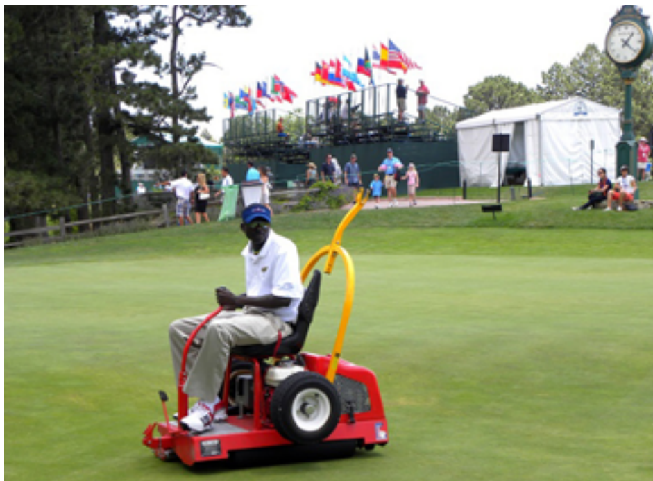
Rollers are becoming more popular for their value in smoothing putting surfaces following aeration and achieving desired green speeds. When the turf is suffering from heat stress in the summer, rolling can even be used periodically as an alternative to mowing because it causes less mechanical injury to the turf.
