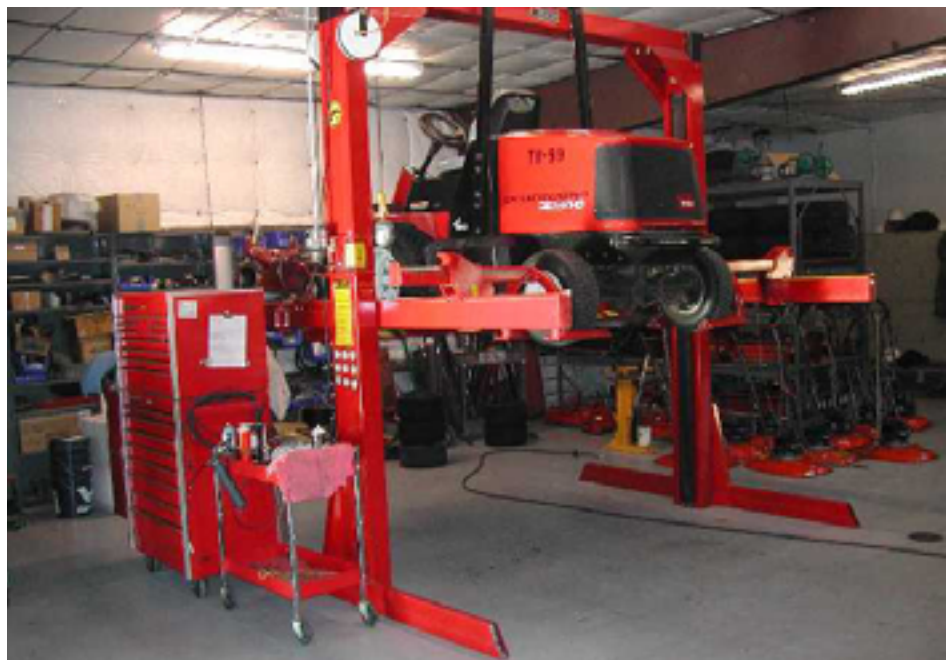
Hydraulic lifts are utilized in the maintenance facility to efficiently service, repair, and calibrate numerous pieces of equipment.
