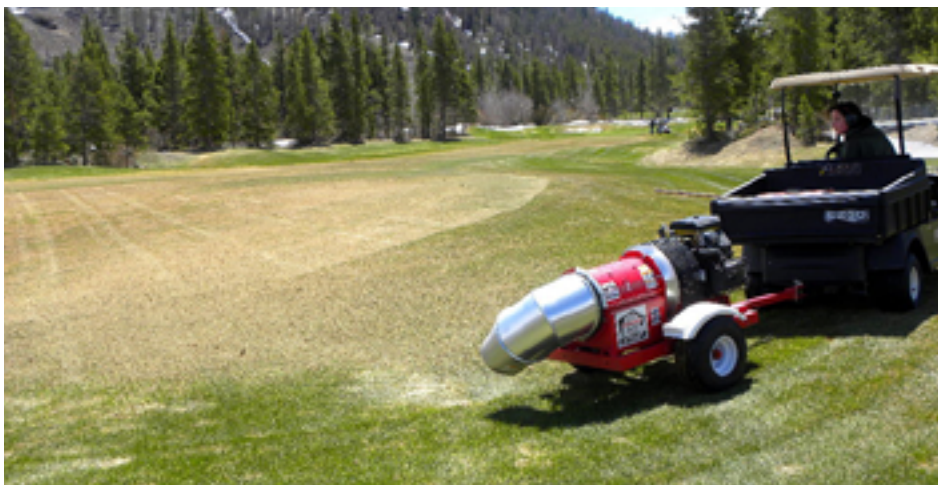
Large pull-behind blowers can be used for debris removal of all kinds around the golf course.
