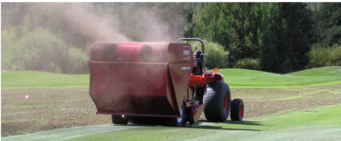
Specialized equipment like this large turf vacuum, or sweeper, can make quick work of clearing debris following core aeration on fairways or in the fall when the time comes for leaf cleanup.
