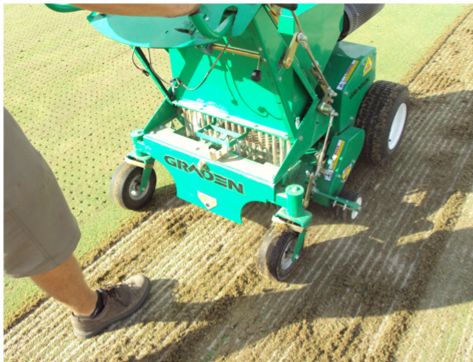
The Graden® Contour Sand-Injection machine simultaneously verticuts and backfills the channels with sand. This machine effectively removes and dilutes organic matter near the surface, but the recovery time could be lengthy.
