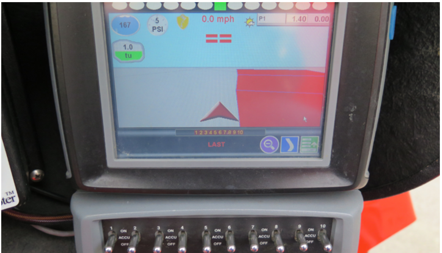
GPS-guided spraying devices allow precise application of liquid nutrients on playing surfaces such as greens, tees, and fairways. This eliminates unwanted overspray and skipping, helping optimize resource use.
