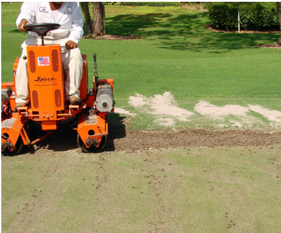
Aeration plugs are sand topdressed, rolled, and kept moist for several weeks while the new perimeters establish.
