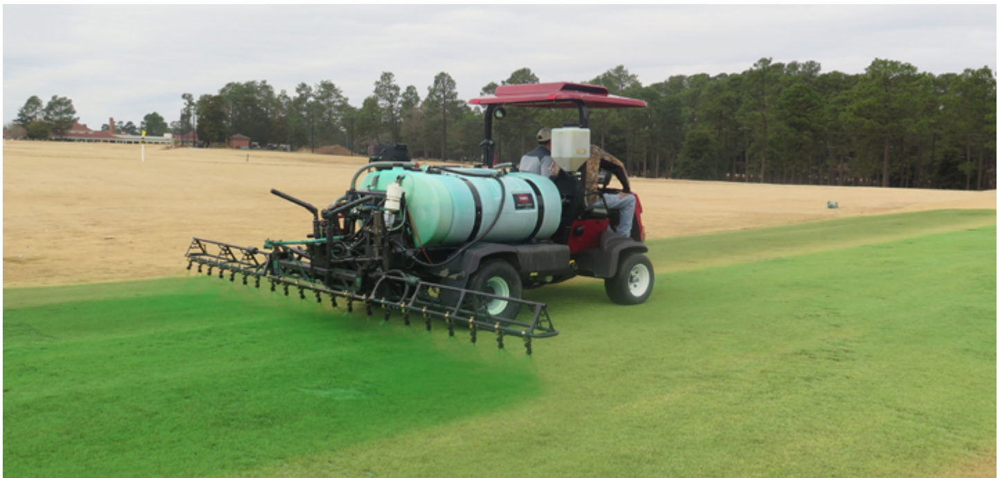
Applying turf colorant using twin flat-fan nozzles spaced at 10 inches apart and a boom height of 14 inches helps maximize coverage and color quality.
