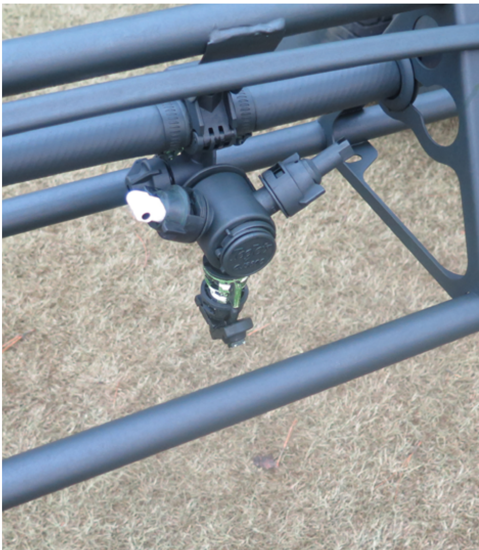
This rotating nozzle body allows course managers to quickly choose between three nozzles, making it easier to use the best nozzle for a specific application.
