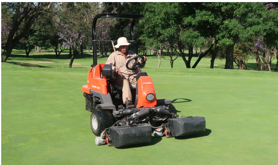
Triplex mowers can provide excellent mowing quality and require fewer employees to mow greens compared to the use of walk-behind greens mowers.
