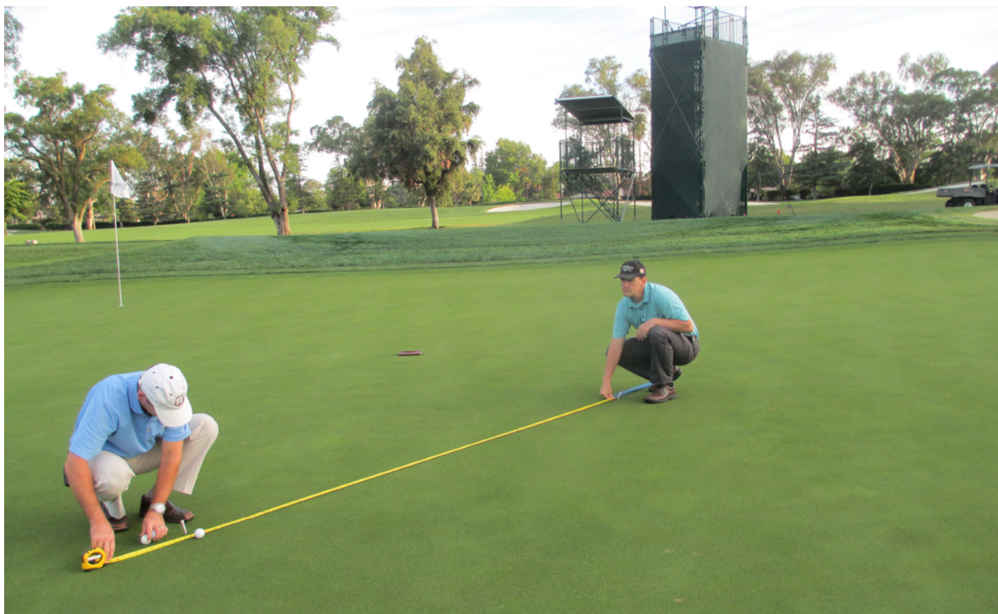
The effects of different cutting heights, mowing frequencies, and rolling will be different for every course. Testing different combinations and taking Stimpmeter readings after each procedure is the best way to determine what works best.
