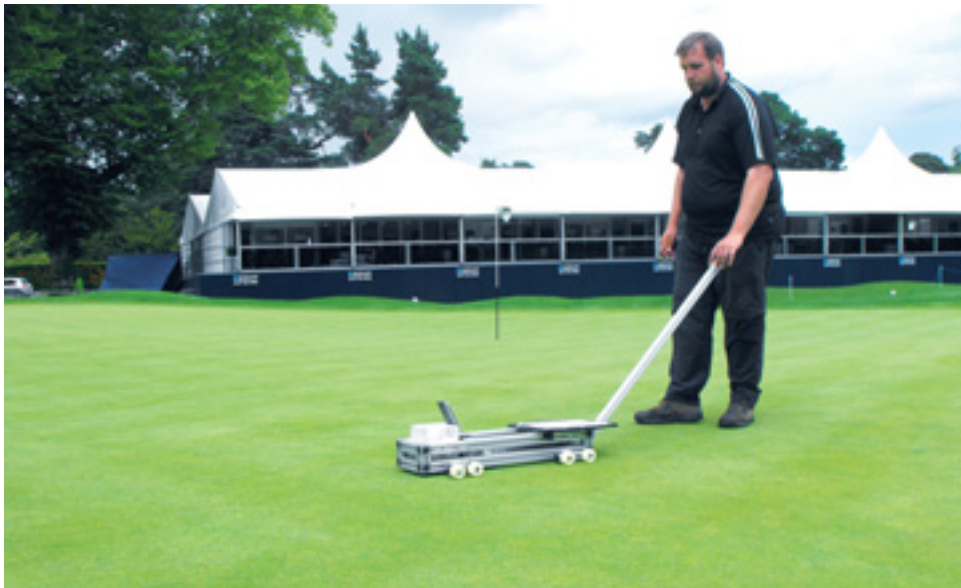
Researcher Dr. Christian Spring measures the smoothness of the putting surfaces at the 2009 Scottish Open at Loch Lomond Golf Club.
