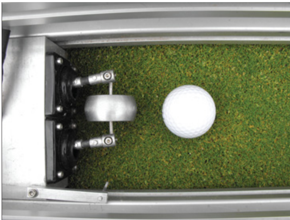
The trueness meter is able to precisely measure the vertical and lateral deviations impacting on the ball.
